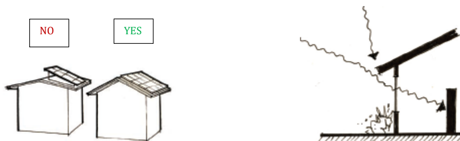
Panels should lay flat on the roof.
